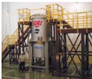
1 GHz NMR unit currently developed by a group of NIMS and Kobe Steel Ltd. The development of this unit, which can achieve up to 920 MHz (21.6 T), is being speeded up so that it can be installed at NIMS located in the Tsukuba Sakura Technopark by the end of this fiscal year.
