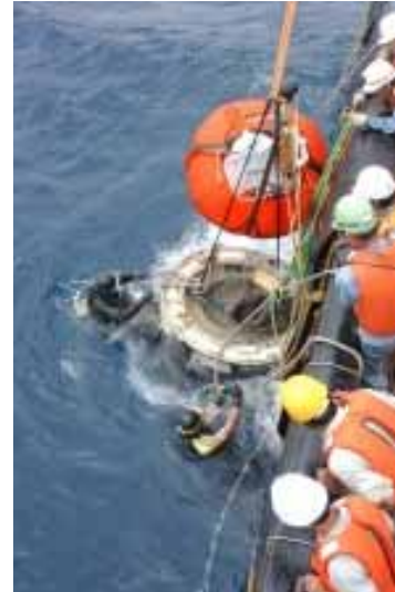
Fig. 2 REV recovery (The REV is under the water below the red floating bag.)
