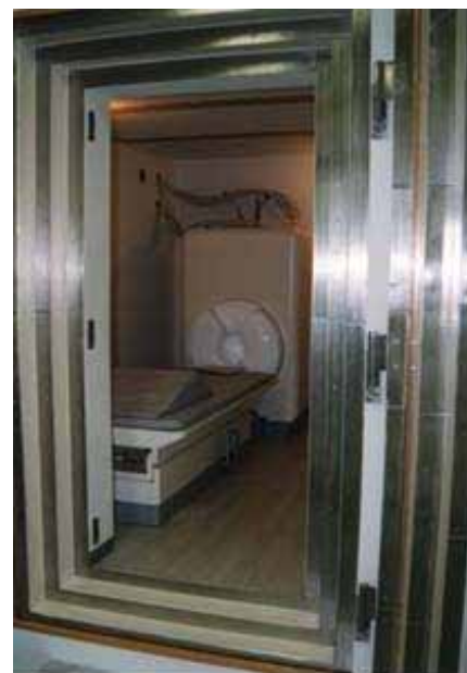
Fig. 2 Dewar and Magnetically Shielded Room
