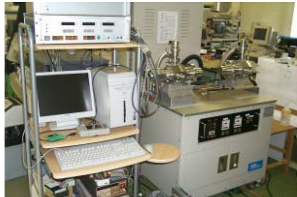
Fig. 2 A magnetic field generator, sold by Aishin Seiki, uses a superconducting bulk magnet. The generator can provide 3T of magnetic field in free space. The development has been jointly carried out by IMRA Material and Nagoya University.
