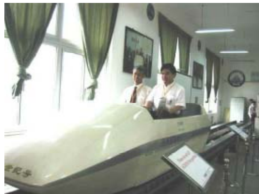
Fig.1 A five-passenger vehicle maglev developed by Southwest Jiaotong University in China. The maglev vehicle installing bulk superconductors levitates above a guide rail made of Fe-Nd-B magnet. (from a Southwest Jiaotong University pamphlet)
