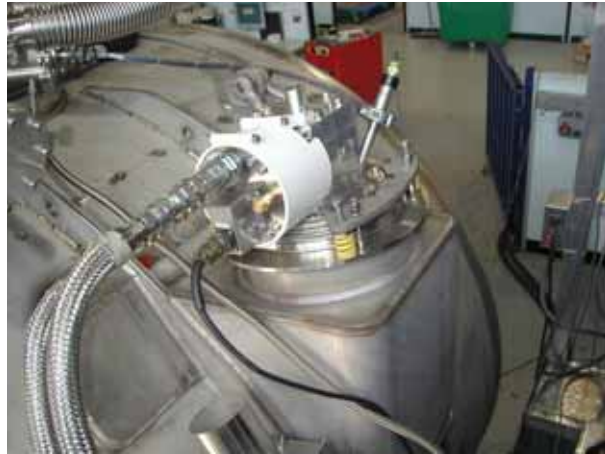
Fig. 3 Magnet with a 4-K GM cryocooler (Cryocooler installed vertically, Siemens)
