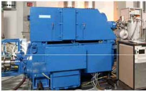
Fig. 2 4 MVA generator for ships (Siemens)
