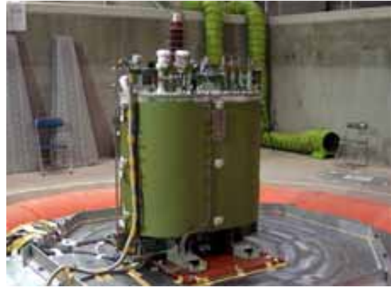
Fig.1 Full-size floor-mounted superconducting traction transformer
