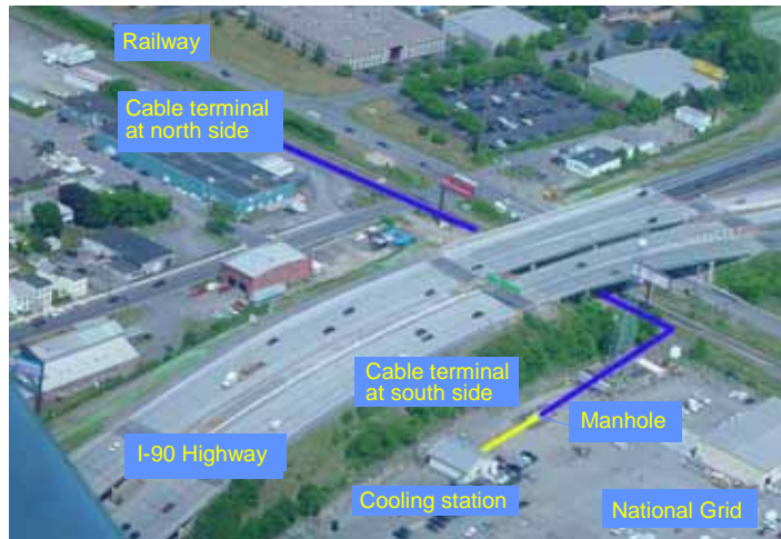
Fig.1 Installation map of high-temperature superconducting cable
