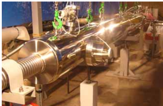
Fig. 3 Three-in-One Joint of three-in-one type high-temperature superconducting cable
