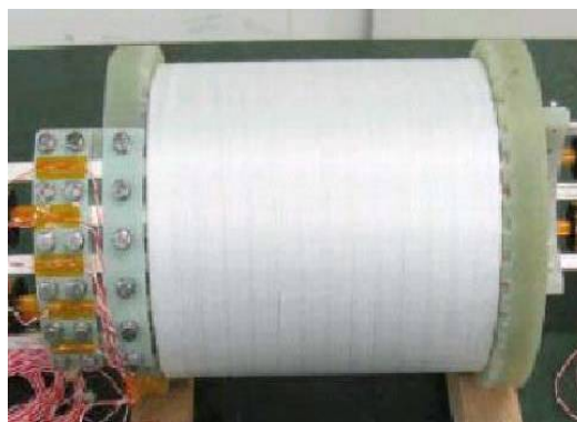
Fig. 1 Model coil of Y-based wires (5-filament 70-m long wire)
