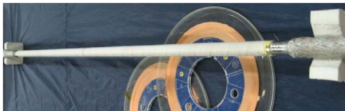
Fig. 2 Appearance of cable core using clad substrate-PLD wire
