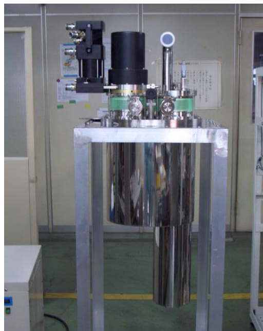
The left half is pulse tube cryocooler and the right half is dilution refrigerator. The length of dilution refrigerator, from the top flange is about 80 cm.
