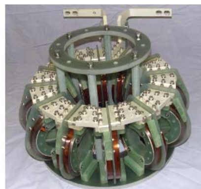
Fig. 1 Appearance of toroid-shape coil using IBAD-MOCVD wires
