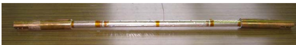
Fig. 3 Appearance of conductor using IBAD-MOD wire
