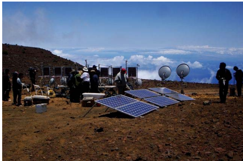
Fig. 4 Power transmission antenna system in Maui Island; this system converts the electricity generated by photovoltaic cells into microwaves and transmits the power from eight small antennas to Mt. Mauna Loa in the far-off distance
