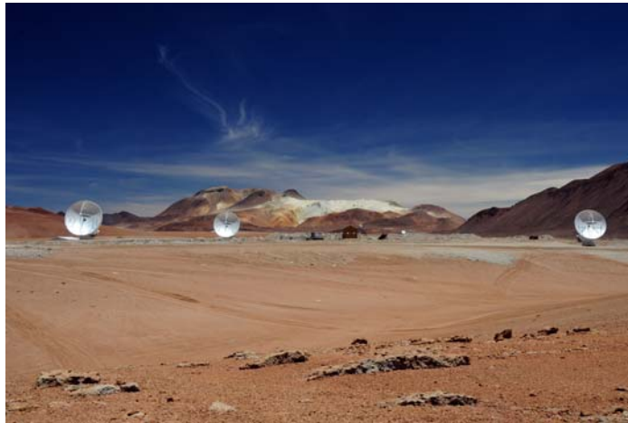
Fig. 1 Three antennas of diameter 12 m installed at the Atacama site, 5,000 meters above sea level. The antenna at the far left is made in Japan.
