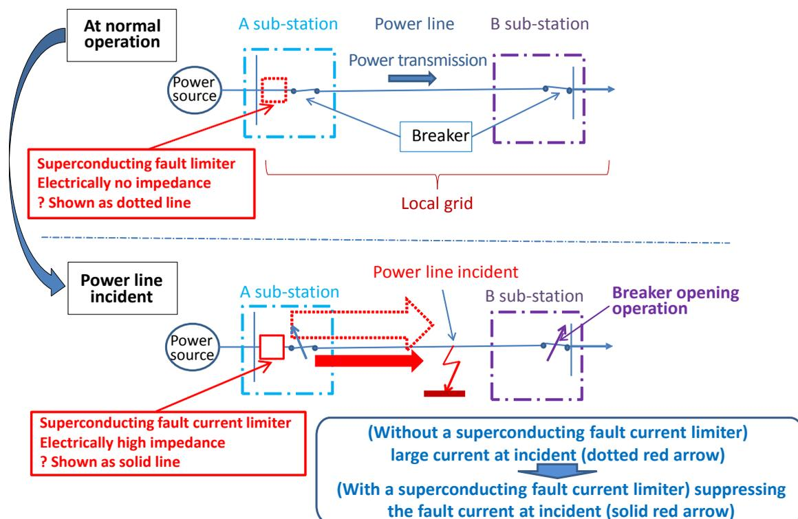
Fundamental concept of a superconducting fault limiter
