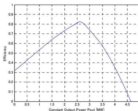
Fig.4 Electric efficiency of ASPCS as a function of the constant output power  $P_{out}$
