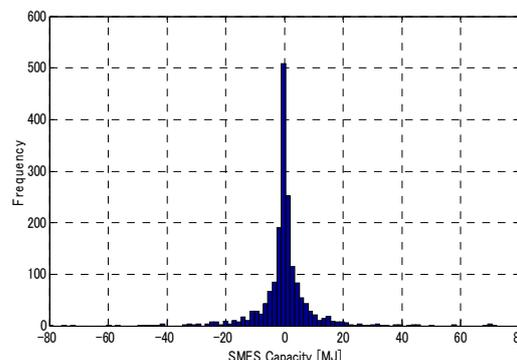
Fig.3 Histogram of SMES input and output energies
