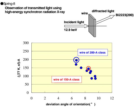
Fig. 2 Relationship between degree of crystal orientation and critical-current characteristics
