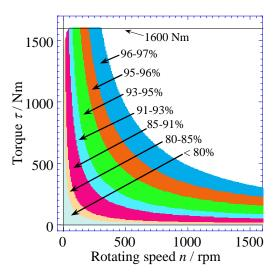
Fig.1 Example of analysis of efficiency map for HTS-ISM of 50-kW class <sup>6)</sup>
