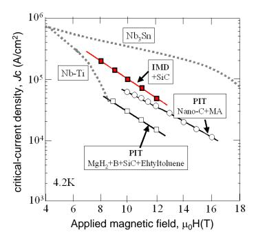
Fig. 2 Representative critical-current density ( $J_c$ )—magnetic field (H) curve of PIT wire<sup>4), 5)</sup> and IMD wire<sup>3)</sup>. Curves of Nb-Ti and Nb<sub>3</sub>Sn are shown for reference.
