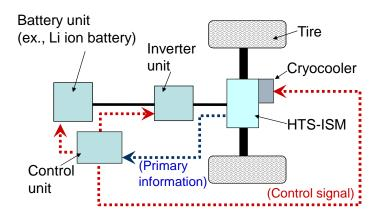
Fig.2 Example of direct-driving-vehicle system provided with HTS-ISM
