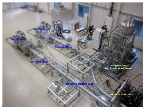
Fig. 1 Layout inside the laboratory
