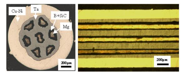
Fig. 1 Transverse section and longitudinal section of  $MgB_2$  wire fabricated by internal Mg diffusion (IMD) method (before heat treatment)<sup>3)</sup>
