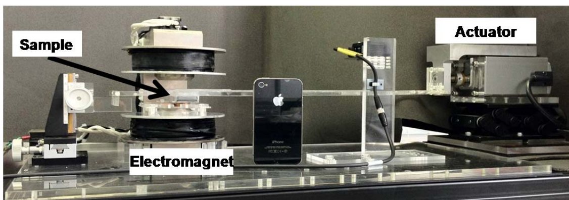
Fig.1 A SQUID DC magnetometer (An iPhone is positioned for scale)
