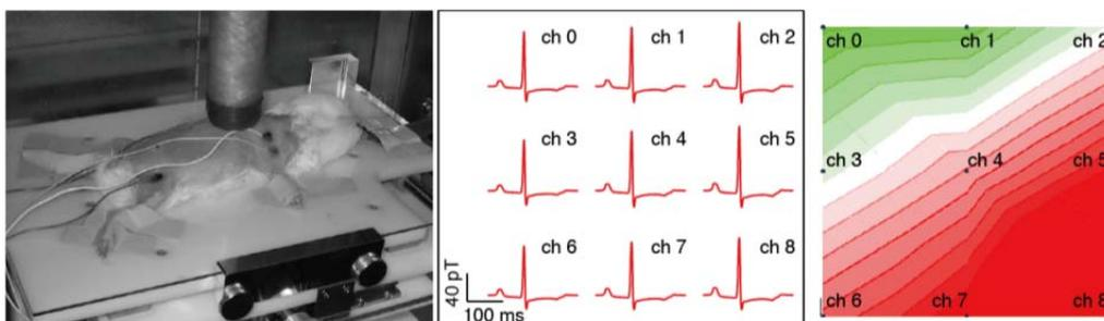
Fig. 3 The set detecting cardiac biomagnetism emanating from a guinea pig (left), Example of MCG signal waveform (center), and the distribution of the MCG signals measured (right). The waveform peaks represent the magnetic field source. On the contour map, the red-areas represent the magnetic field source whilst the green represents the magnetic field sink. The distance between the contour lines is 300 ft.
