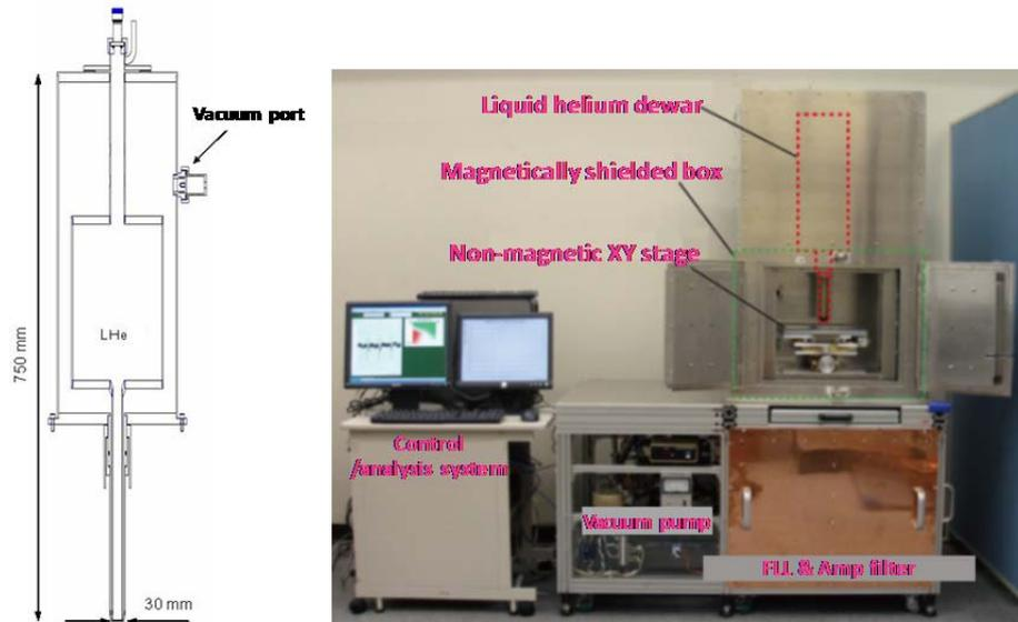
Fig. 2 Structure of a suspended dewar (left) and the overview of the MCG system designed for small animals (right)
