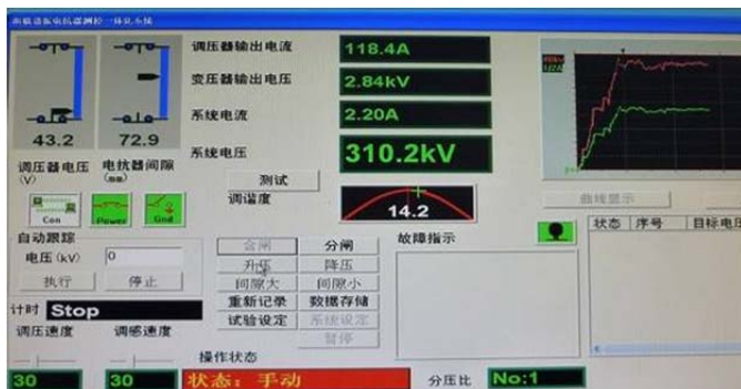
Fig. 4 Screen and partial discharge signal of current transformer at partial discharge test
