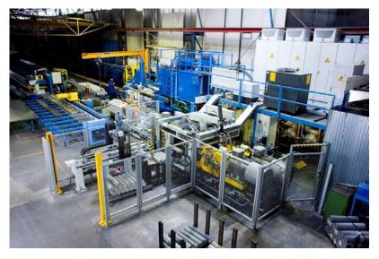
Fig. 2 Superconducting furnace system currently in operation. Continuous operation without the awareness of superconductivity.
