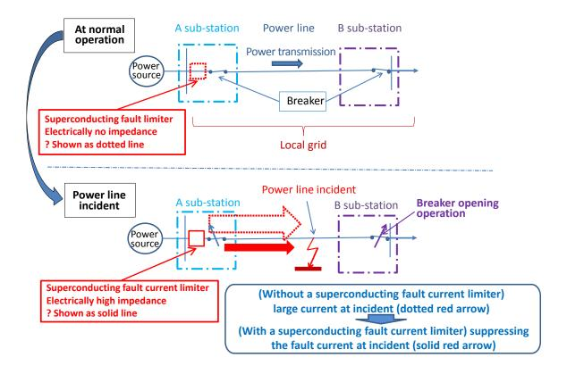
Fundamental concept of a superconducting fault limiter
