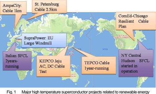
All are grid demonstration trials, except SupraPower-Pj (wind power). SFCL: Superconducting fault current limiter
