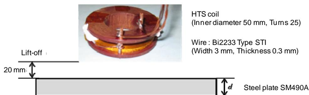
Fig. 1 Measurement of steel plate thickness utilizing HTS coil
