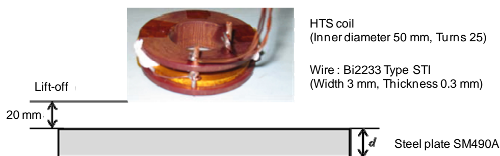
Fig. 1 Measurement of steel plate thickness utilizing HTS coil
